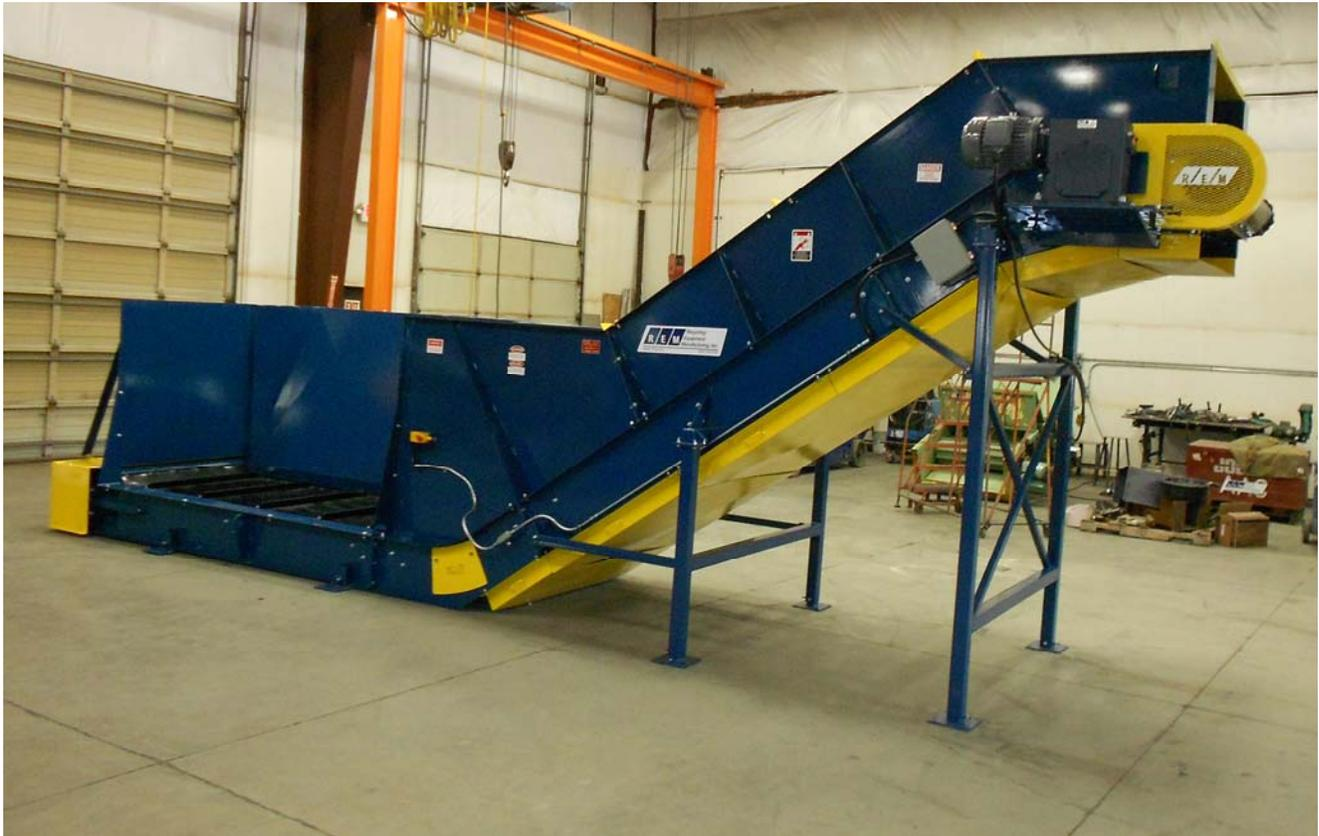
REM® offers a wide variety of equipment to meet the needs of many different industries. The “Low Profile” feed conveyor was designed to provide an easy to load conveyor without the cost of installing a pit into your facility. With the heavy duty low profile conveyor you are able to bulk feed above ground with no need for pit installation. This allows for a higher feed rate for your baling operation.
